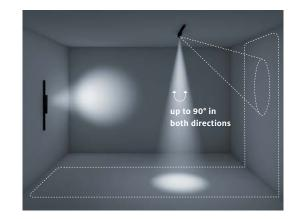
SUPERSYSTEM integral pivotable downlight Blind cover | 3-phase track | surface-mounted
