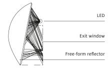
Technical highlight: The patented liteCarve® free-form reflector creates a rectangular cone of light from a round half disc. Homogeneous and perfectly glare-free.
