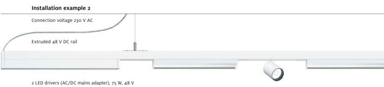
Input to both ends of the rail; no electrical connection in the centre of the rail
