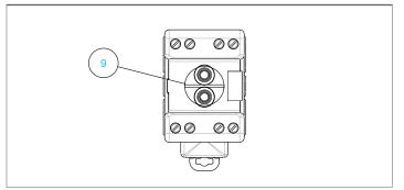
If the actuating element being fitted is a position selector switch, make sure its actuating pins are in alignment over the metal plungers on the switch module (9).
