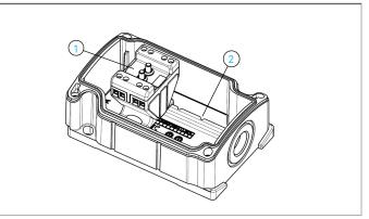
Snap the devices (1) onto the rail of the enclosure (2) with the latch positioned in the cut-out in the rail. Please see manuals of Exchange modules.
