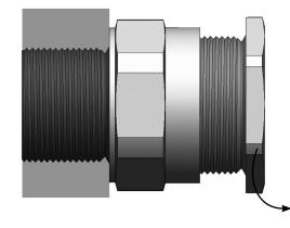
5. Pass the cable through the gland to the desired position, then tighten the seal nut by hand until resistance is felt (when the seal contacts the cable). Tighten with a spanner one further turn.
