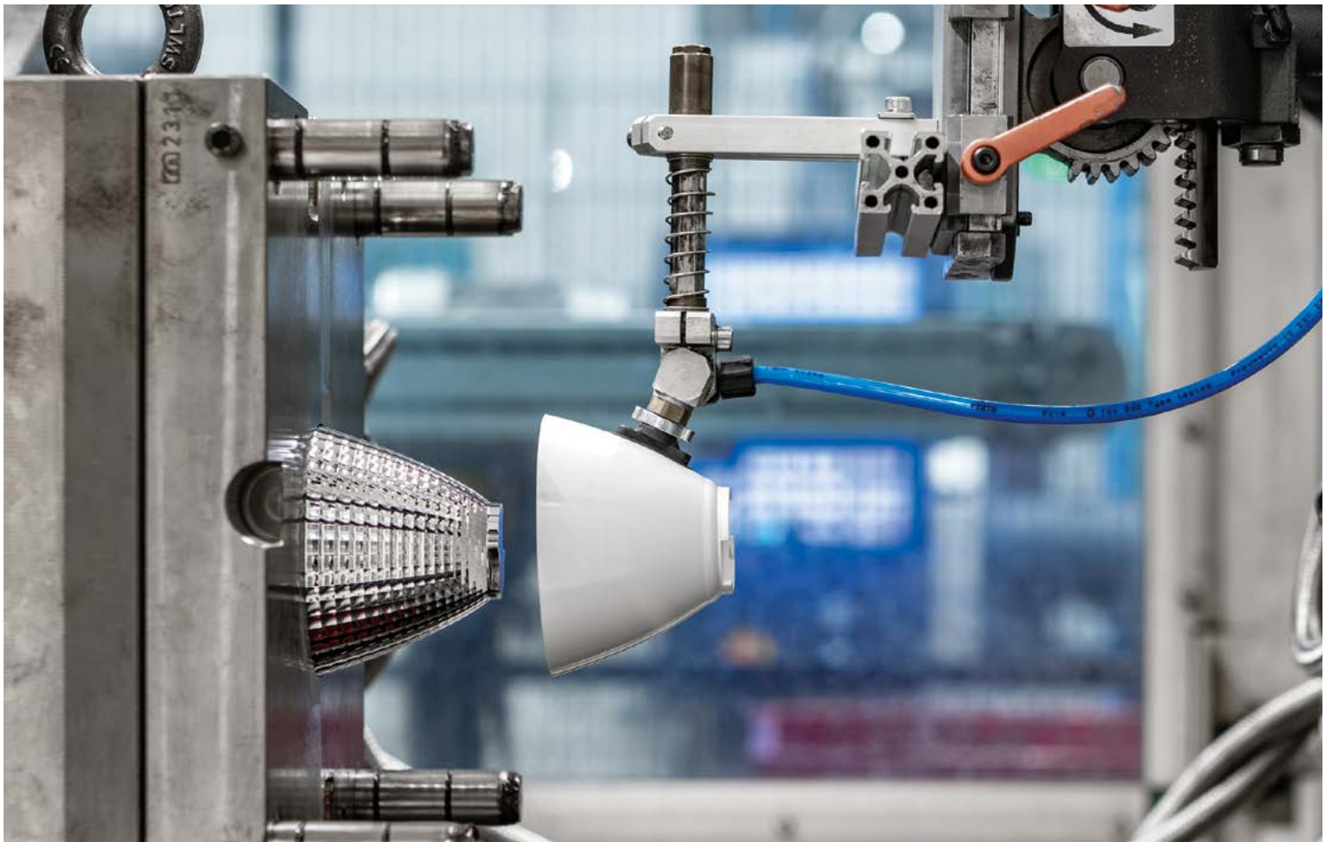
Highly efficient, injection-moulded reflectors with sputtered finish, designed and manufactured by Zumtobel in Germany
