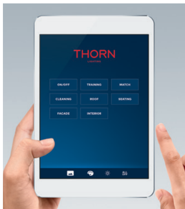
Lighting playback controller with touch panel (in-or external)
